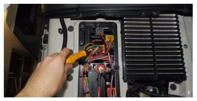
1. Find wire number 7004 (CAN High) and 7006 (CAN Low) located on the front of car, Like on the photo.
