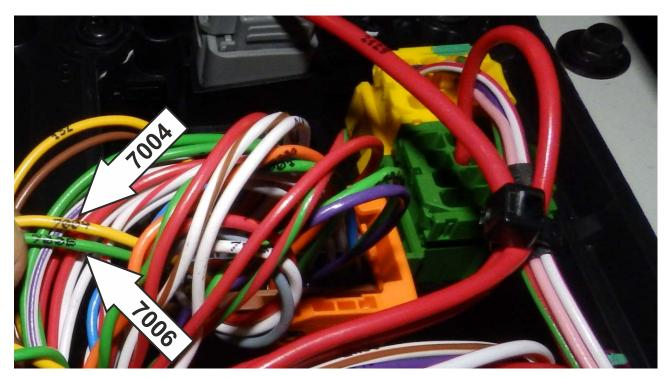
2. Connect wires from the emulator as follows: YELLOW wire from emulator ---> 7004 (CAN High) GREEN wire from emulator ---> 7006 (CAN Low)
