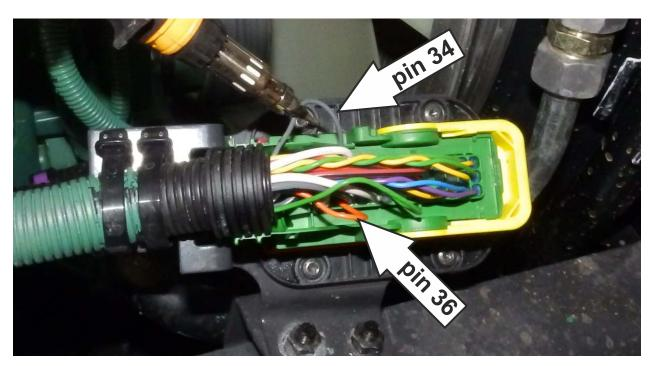
4. Connect wires from the emulator (two long wires in a black isolation) as follows:
