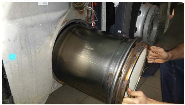
6. You should disconnect plug from the pump and remove DPF. If car have any errors, remove them from ECU
